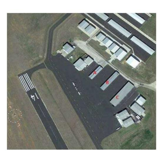
The County owns 3 t-hangars that can support 20 small aircraft. They are fully enclosed with sliding doors. The majority of the facilities are "open bay" with limited electrical access. Access to the hangars is from the north ramp and the facility has quick access to the runway.
